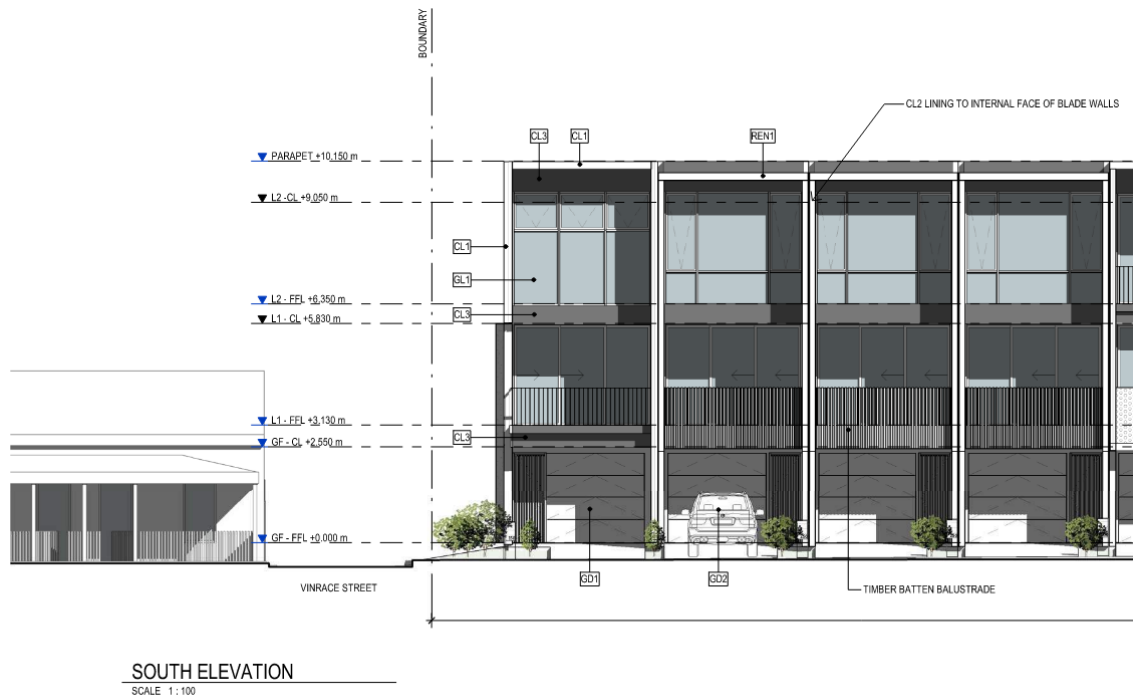
Figure 1: Proposed south elevation of townhouses on Vinrace Street with the subject site visible on the left.
